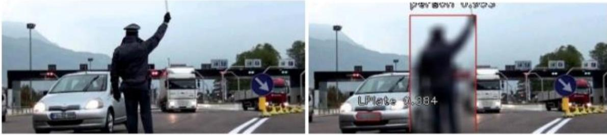
Figure 5: An example of applying the Complete Algorithm for anonymization to an input image (on the left side) containing two of the classes of interest: *license plate* & *person shape*, respectively.
