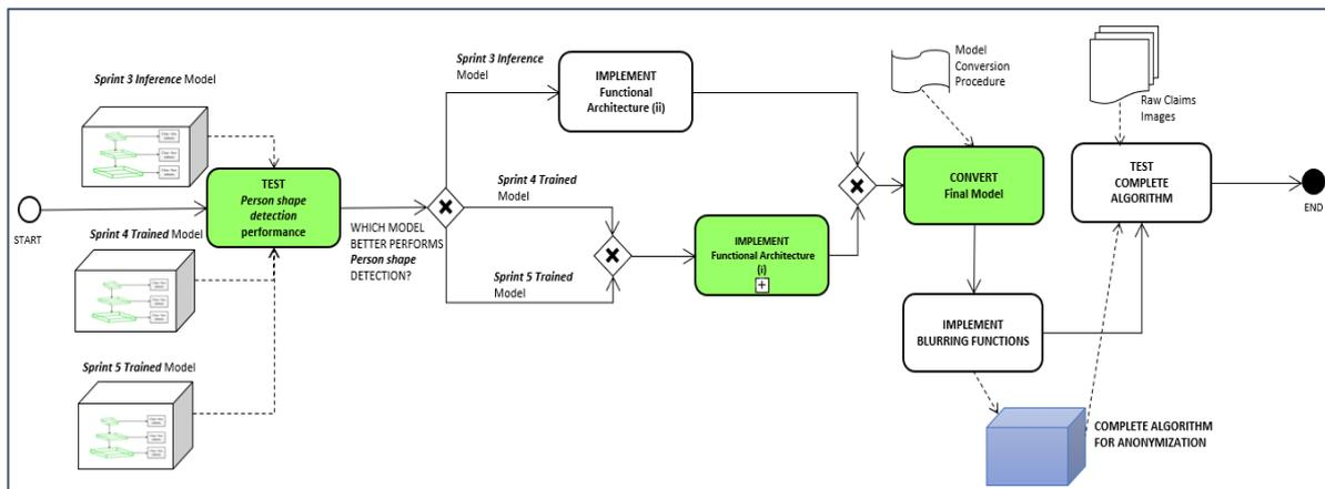
Figure 3: Decision flow diagram regarding the steps carried out by the project team during Training and Validation of the Object Detection algorithm project phase. In green, it is highlighted the effective decision-making process followed by the project
